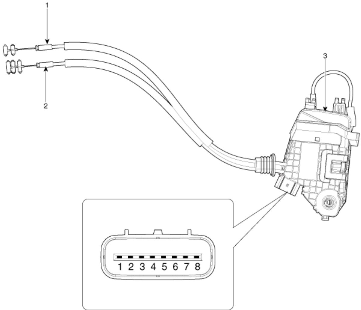
1. 门锁闭锁/开锁机械操纵钮拉线
